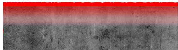
Silicate coatings penetrate into the substrate and form inseparable chemical bond
